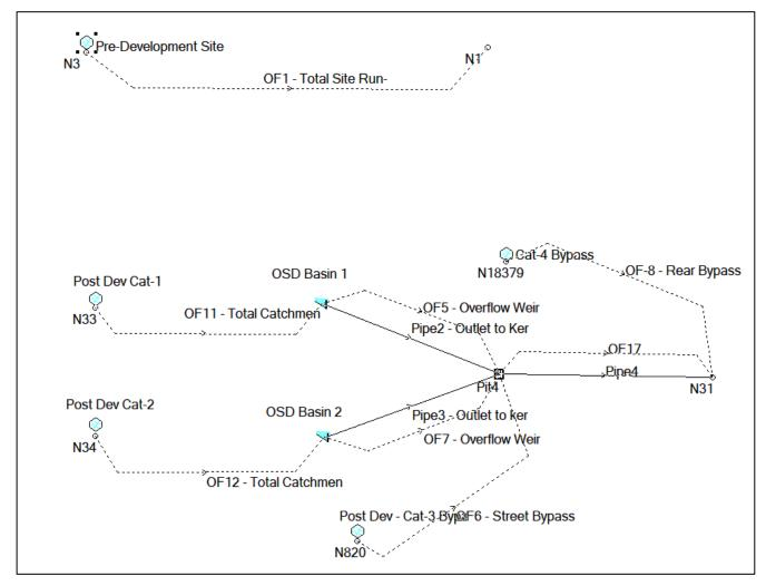
Overall set up of DRAINS Model
