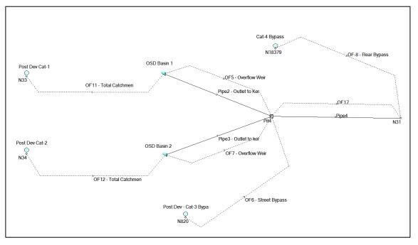
Figure 3 – General Arrangement of Post Development Drains Model
